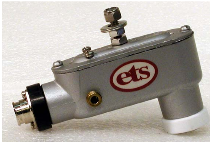
Figure 2.1-2: Standard Charged Plate Detector Sensor
