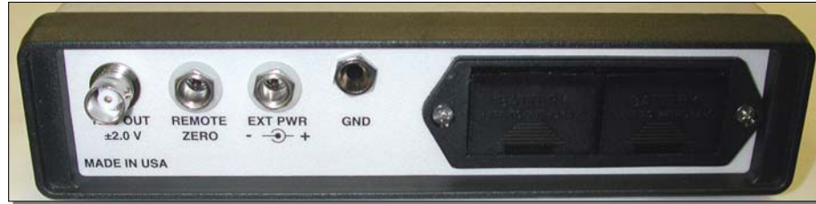
Figure 2.0-2: Model 230 Nanocoulombmeter rear panel
