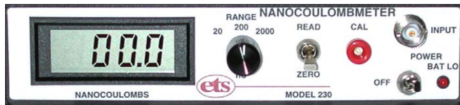
Figure 2.0-1: Model 230 Nanocoulombmeter front panel
