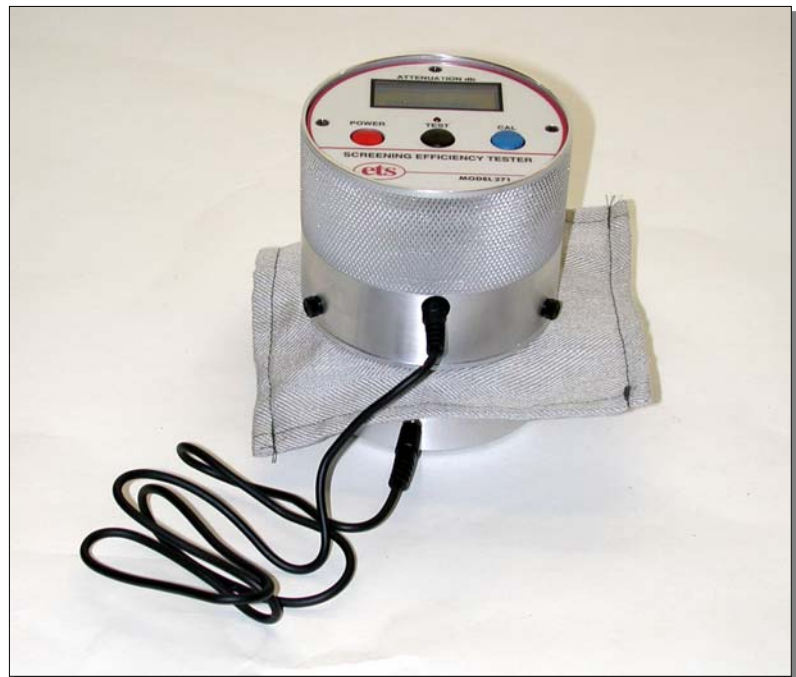
Figure 1 Model 271 Screening Efficiency Tester
