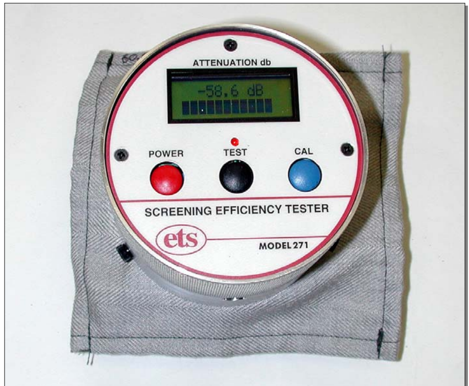
Figure 2 Measuring screening efficiency
