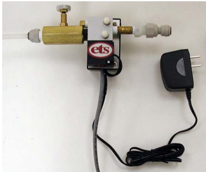
Figure 2.2-1 Control/Solenoid/Flow Regulator unit
