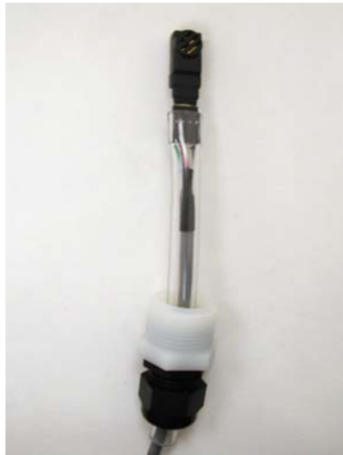
Figure 2.1-1 Sensor mounted in compression fitting
