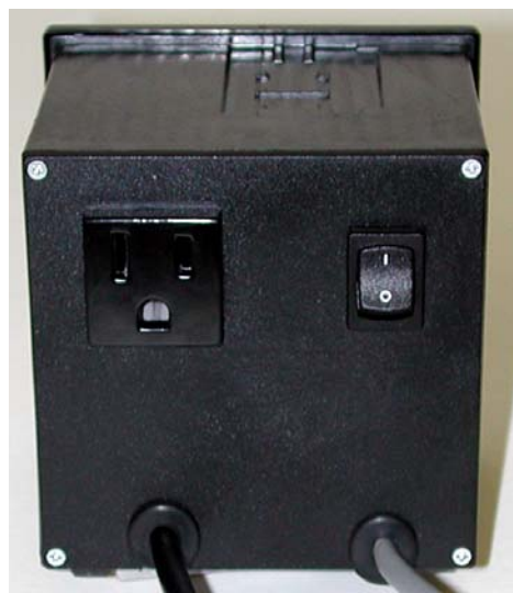
Figure 3.2-3: Control Unit rear panel
