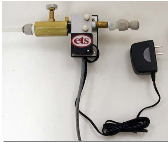
Figure 3.1-2: Control/Solenoid/Flow Regulator unit
