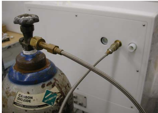
Figure 4.0-1: CO 2 cylinder hook up
