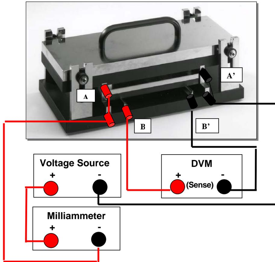
Figure 1.0-2: Model 831 meter connections
