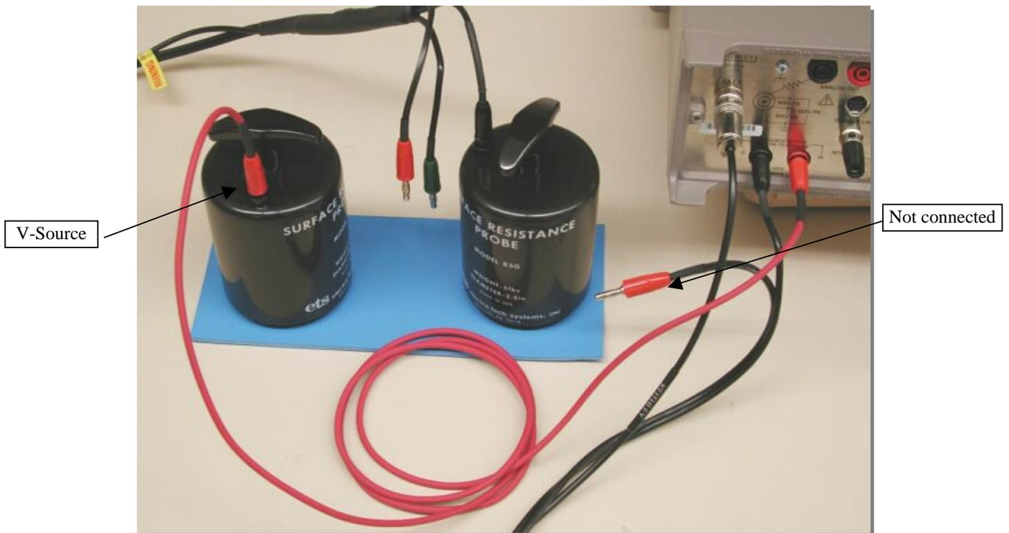
Figure 2.0-4: Point-to-Point Resistance
