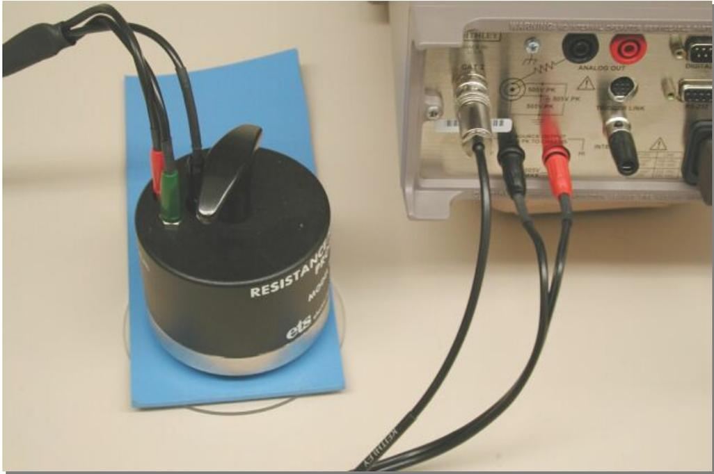
Insulating Plane is used when measuring static dissipative materials per ESD S11.11
