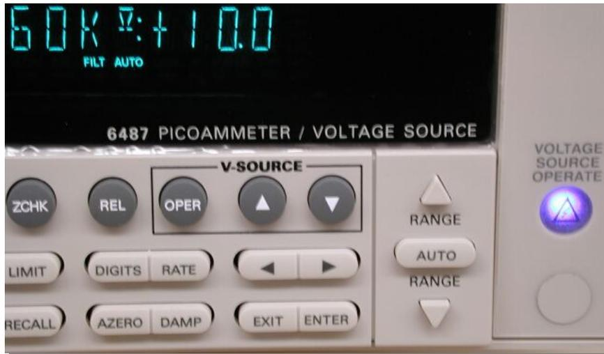
Figure 4.1–1: Source Voltage Adjust
