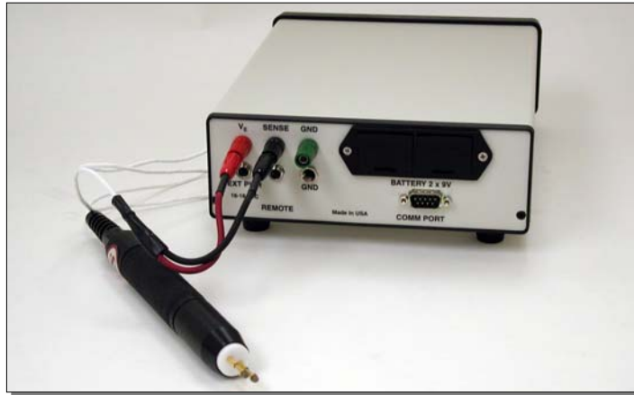
Figure 3.1-3: Connection for measuring 2-point resistance per ESDA STM 11.13
