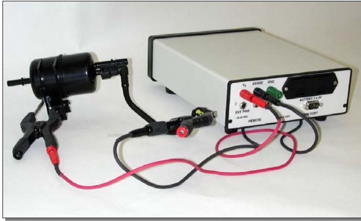
Figure 3.1-5: Connection for measuring point-to-point resistance per SAE J1645
