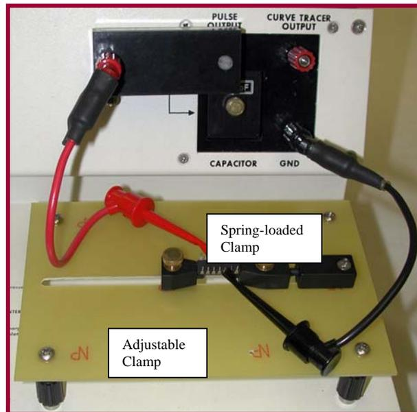
Figure 3.0-3: Universal Clamp Test Fixture (HBM)
