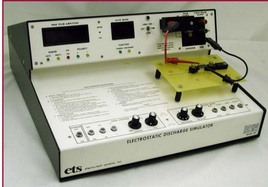
Figure 2.0-1: Model 910 ESD Simulator (with optional CDM)
