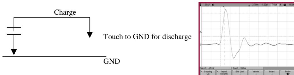
Figure 5.0-3: Basic Charge Device Model equivalent circuit
