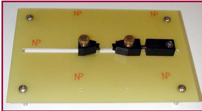
Figure 2.0-2: Standard universal DUT holding fixture
