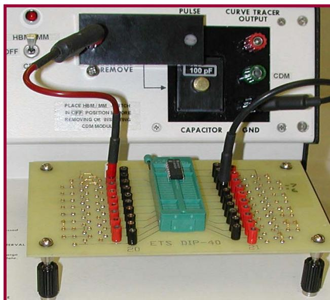
Figure 3.0-4: 40-pin DIP Socket Test Fixture (HBM)
