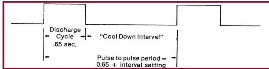
Figure 2.0-5: Automatic Mode Timing Cycle
