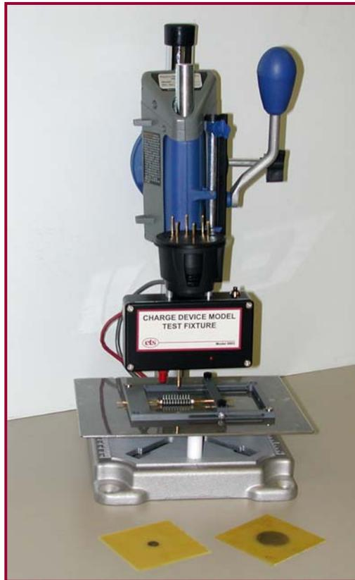
Figure 5.0-4: Model 9903 Charge Device Model Test Fixture
