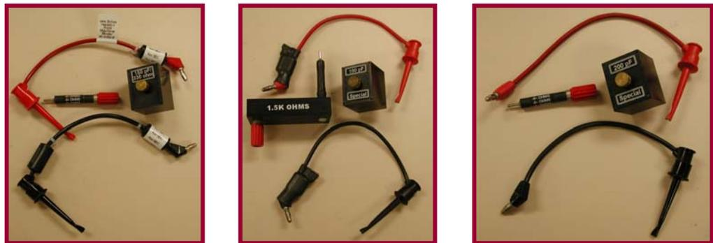
Figure 3.0-2: IEC 61000-4-2 RC network module and HBM & MM Special
