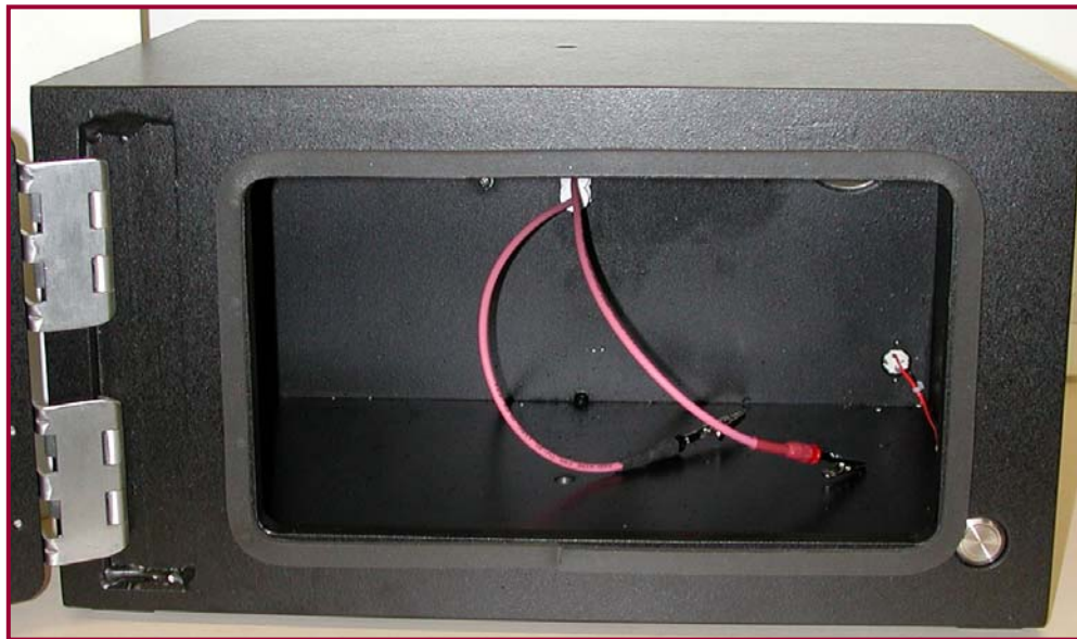
Figure 2.4-1 Firing Test Chamber with discharge cable
