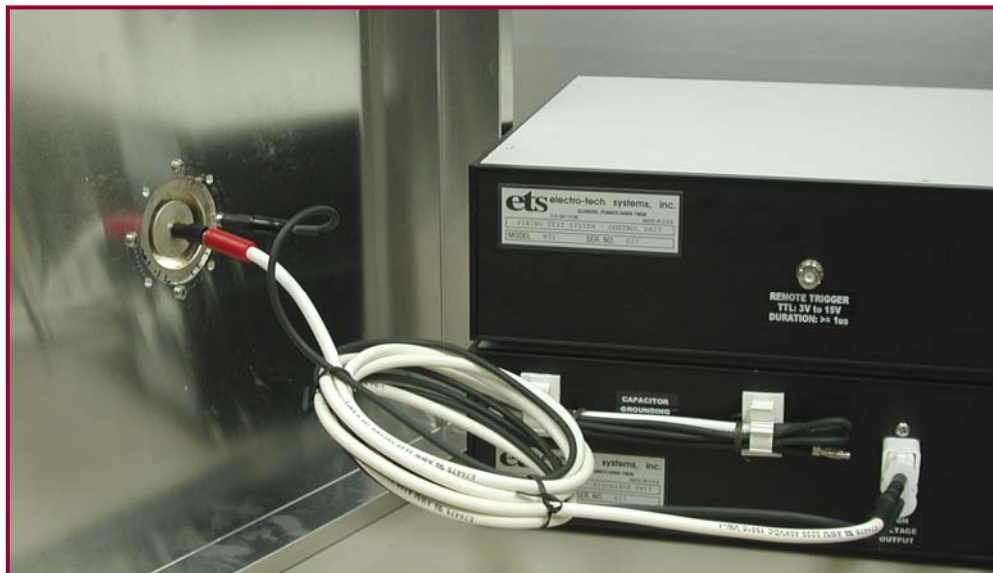
Figure 6.0-3a: Current pulse calibration set-up, external Test Target
