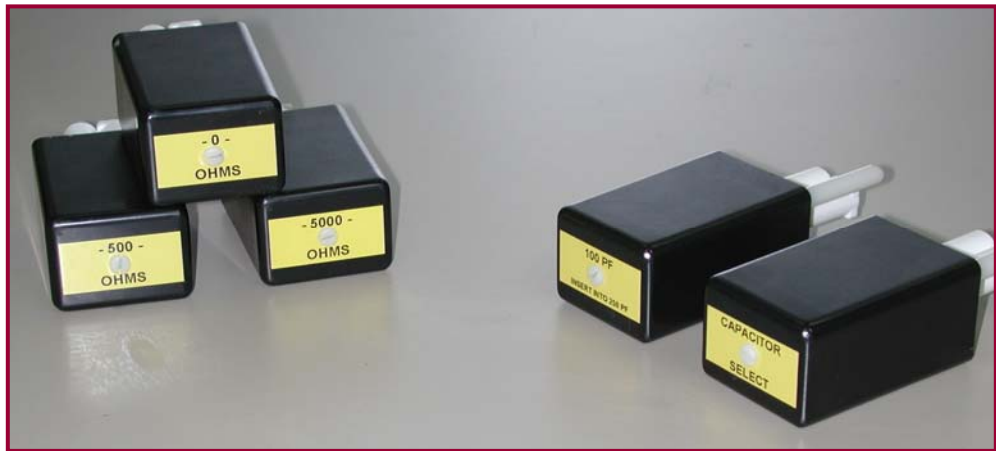
Figure 2.2-2: Standard selector and R/C modules
