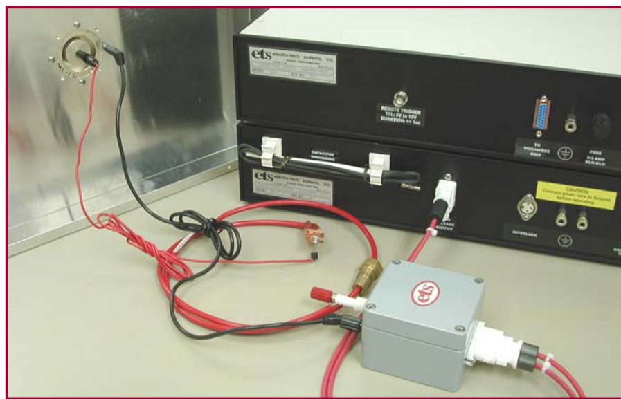
Figure 5.0-3: Typical current monitoring test setup with Junction Box
