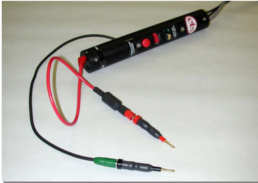
Figure 3.0-6: HBM test set up using external leads
