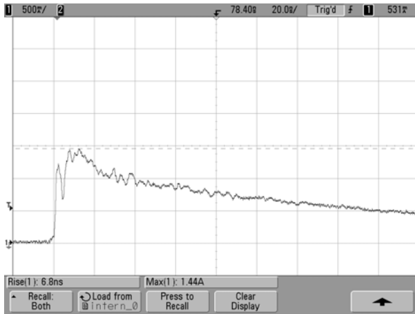
Discharge using 12" leads
