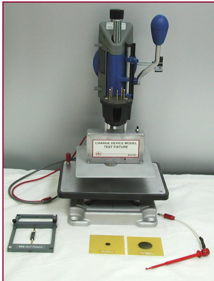
Figure 6.0-4: Model 9903 Charge Device Model Test Fixture
