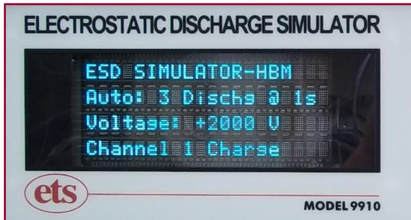
Figure 3.0-2: HBM testing in Auto mode at +2000V
