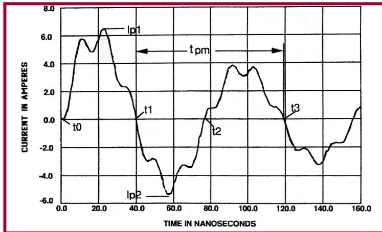
Figure 5.0-7: Current waveform through a short to ground
