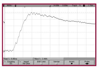
Figure 5.0-4: Model 9910 Rise Time and Ringing Waveform at 4kV
