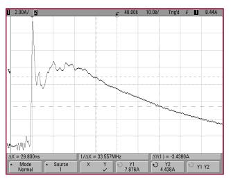
Figure 5.0-11: Actual Model 9910 HMM waveform at 4000V.
