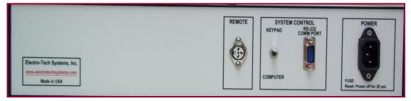
Figure 2.0-5: Rear Panel (standard configuration)
