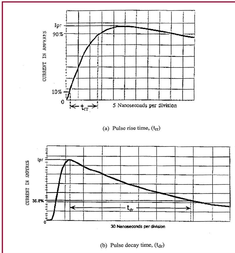
Figure 5.0-6: Current waveform through a 500 Ohm resistor
