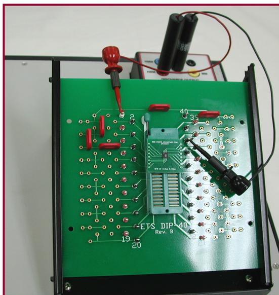
Figure 2.0-8: 40-Pin DIP DUT Board with programming pins
