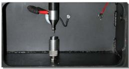
The Model 949 Test Target is a current transducer with  $50\Omega$  impedance and frequency response to 1 GHz that is used to measure all ESD output waveforms. It has a transfer ratio of 1 Volt/amp. A 3' (91cm) RG58 cable is included. The Model 949 is designed in accordance with IEC 61000-4-2
