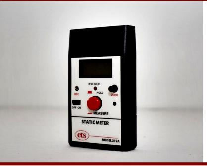
Accurately measures the magnitude and polarity of electrostatic fields. The Electro-Tech Systems Model 212 is a lightweight, convenient handheld unit that allows quick assessment of electrostatic fields or the charge on objects.
