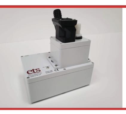
**Electro-Tech Systems Humidifier is** built for industrial and laboratory applications. The 5482 is a high-performance humidifier with dual-rate operation, automatically choosing fast ramping when required, or lower rate operation to precisely maintain a target condition. The unit creates a 5-micron droplet size which avoids moisture deposition on sensitive items. The 5482 functions with any ETS series 5200 controller.
