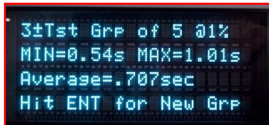
Figure 6-10: Display when new group can be entered (Cutoff is changed or Auto count is changed)
