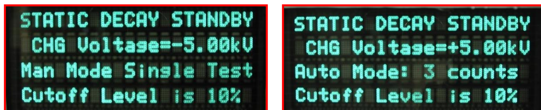
Figure 2.2-2: Static decay display in ZERO/STBY mode
