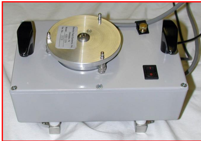
Figure 7-6: Nondestructive Static Decay Test Fixture
