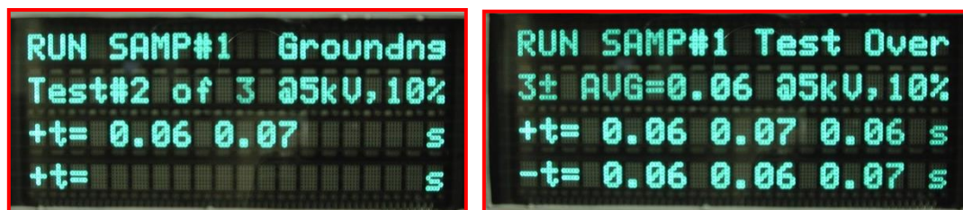
Figure 2.2-7: AUTO mode decay time measurement
