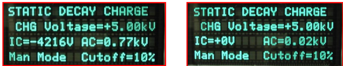
Figure 6-1: Sample with and without IC and very low AC
