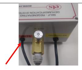
Step 3 – AC supply for circuitry Power cord #1 is on the left. This power source stays energized at all times, Power is supplied to the air dryer, (100VAC to 240VAC, single phase, 50-60 Hz)
