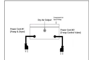
Step 1 – Dry Air Output The dry air output is located on the rear, center of the unit (with 1/4" Quick Connect fitting and a flow regulator).
