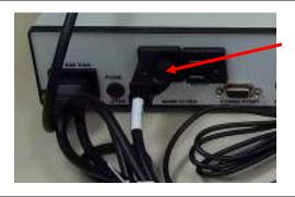
Step 5 – Controlled AC power source This AC line cord is normally plugged in to the RH DECR outlet of a controller to dry the chamber.
