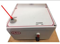
Step 6 – Connect Air Source. Connect a Compressed air source to the air input fitting on the top of the enclosure. Regulate compressed air to 50 to 100 PSI.
