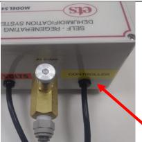
Step 4 – Controlled AC power input Power cord #2 is on the right. The AC power (100VAC to 240VAC, single phase, 50-60 Hz), is to be connected to a controlled AC circuit (see below). When power Is applied, dehumidification takes place.
