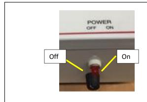
**Step 1 --** Turn the Power ON. Turn the power switch on the front panel to the right, or "ON" position. The dryer will begin operating immediately to produce dry air. Some sounds will be made by the mechanism – this is normal.
