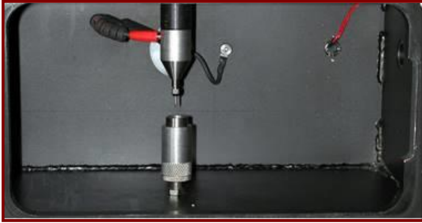
Figure 6.8 Powder discharge and sample holder assembly.
