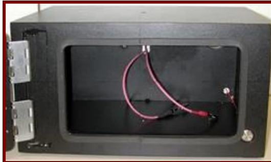
Figure 6.7 Firing Test Chamber with discharge cable.
