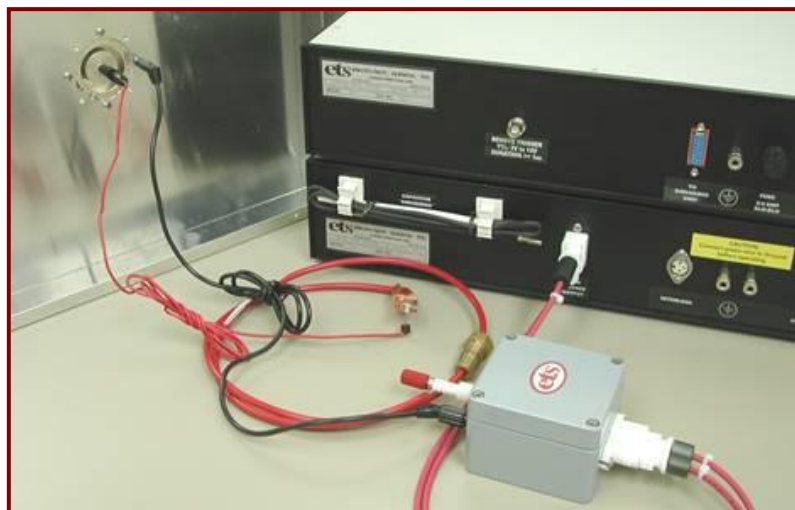
Figure 4.3 Typical current monitoring test setup with Junction Box
