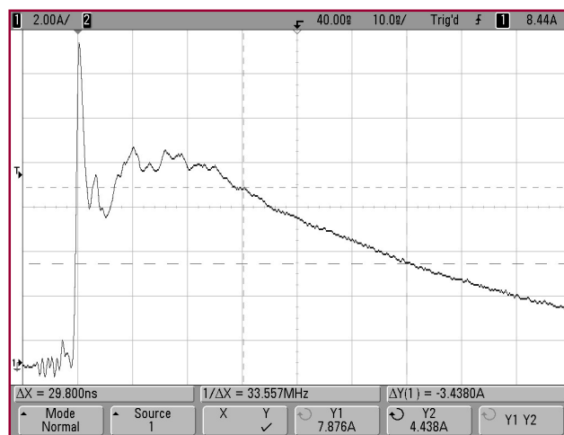
Figure 5.0-11: Actual Model 9910 HMM waveform at 4000V.
