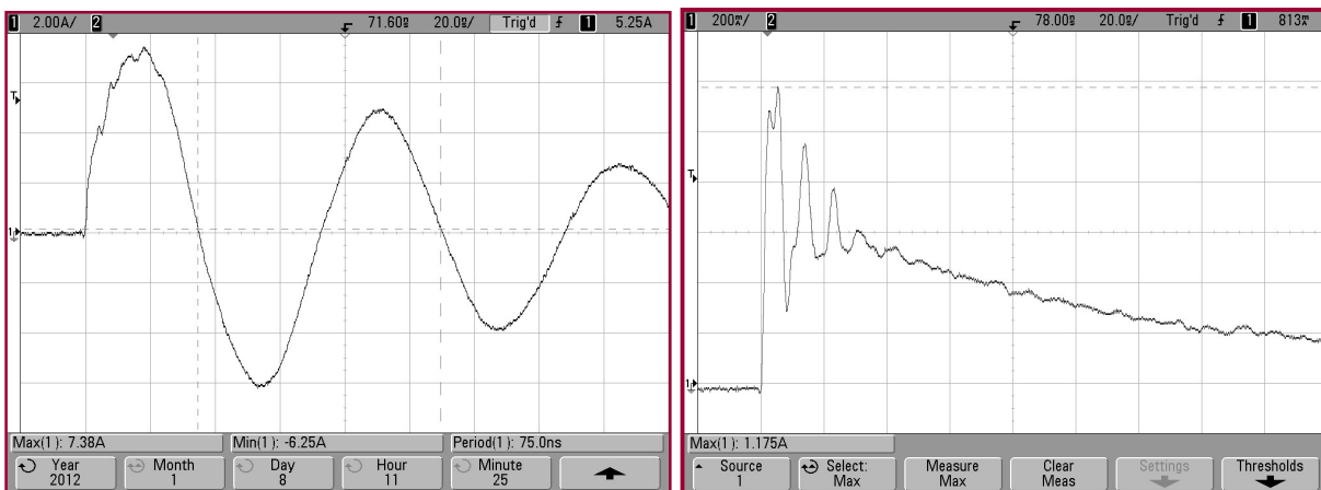
Figure 5.0-8: Current waveform through a 500 Ohm resistor to ground
