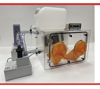
Electro-Tech Systems' 5504 is a compact benchtop chamber offering a working space of 3.25 Cubic feet (92 Liters). The 5504 can be configured as basic glovebox or, when integrated with ETS operating systems, an environment with complete humidity & temperature control. Its clear acrylic construction provides you with complete visibility. Offered in a variety of packages the 5504 is the ideal glovebox for small applications with critical environment requirements.
