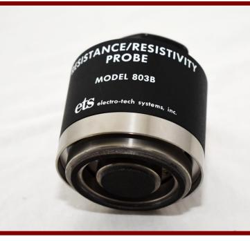
Evaluate your material's surface and volume resistance and resistivity characteristics. Electro-Tech Systems' 803 delivers critical insight on these metrics for planar surfaces. The electrodes are made from a conductive silicone for excellent probe-to-test-surface contact which allows measurements of 100 Ohms and greater to be made. The 803B comes complete with metal and acrylic test beds and is compatible the recommended Model 871 Wide Range Resistance Meter.
