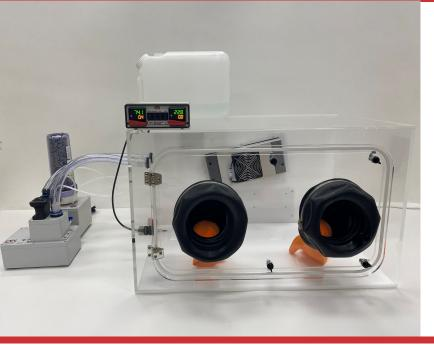
The M 5507 midsize glovebox chamber creates a controlled, sealed environment for critical lab and industrial processes. Its flexible control system empowers you to configure temperature and humidity with precision, tailoring the chamber to your exact needs.
