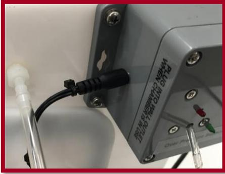
**Step 6.D Verify Overpressure Sensor is set up correctly.**
