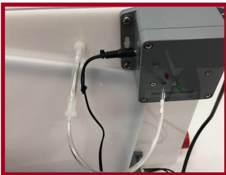
**Step 6.C Verify Overpressure Sensor is set up correctly.**
