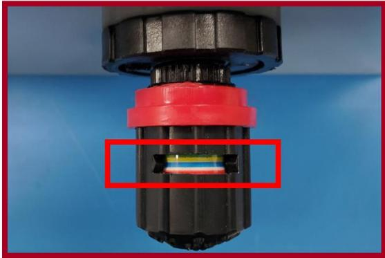
**Step 7. Verify Flow Control is in Correct Position**
