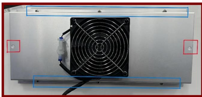
Use two 8-32 X 3/4" screws which goes on the left and the right side of the thermoelectric unit (indicated in red) which will mount the thermoelectric unit on the chamber securely. There should be about minimum of 6 inches (recommended 1 foot) gap between the thermoelectric unit and anything behind it to prevent restricting of the airflow.
